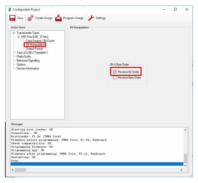
Binary number after load will be readed conversely /reverse, bit by bity ( don't forget for 9 bits to 37b ):
